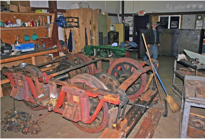
A view of a Climax truck rebuild shows new parts, such as the brake beam, and extensive weld repairs.
