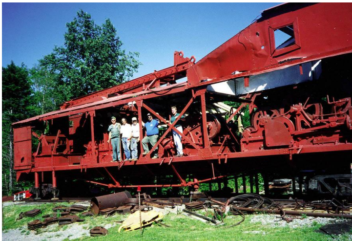
The skidder in place at Camp One showing the three winch engines used for raising the tower and actual skidding operation. Original plans were to erect the 85-foot tower, and ground anchors were prepared for the guy wires and stays, but we could not get engineering approval from the state, so the tower remains displayed horizontal on the ground.
