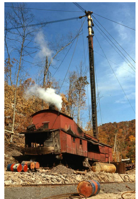
The skidder in place at Camp One showing the three winch engines used for raising the tower and actual skidding operation. Original plans were to erect the 85-foot tower, and ground anchors were prepared for the guy wires and stays, but we could not get engineering approval from the state, so the tower remains displayed horizontal on the ground.
