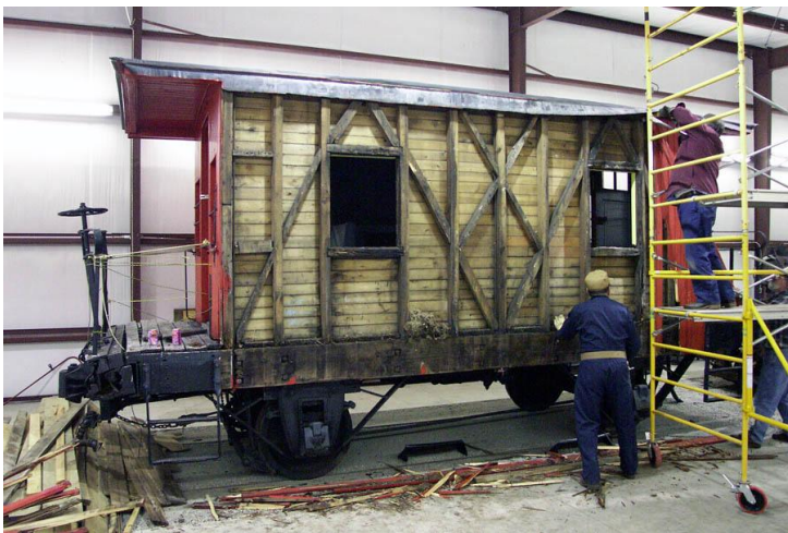
An early Cass acquisition was the ex-Elk River Coal & Lumber Co. bobber caboose dating from the 1880s. Used frequently at Cass from the 1960s, but 40 years later, needed a rebuild. MSR&LHA accommodated, rolling out the completed product in 2003.
